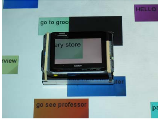
Figure 36 Synchronization between handheld and DiamondTouch table
